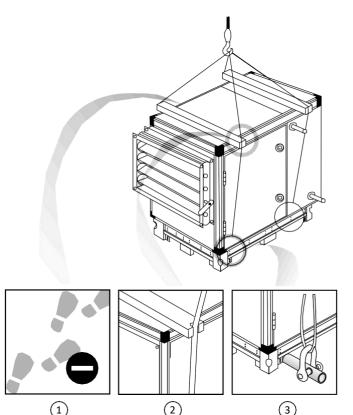
Figure 1 - Crane operation procedure
