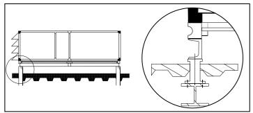
Figure 6-1: Foundation construction on steel supports by others
